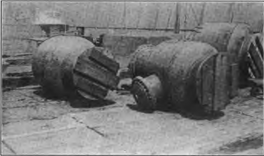
FIG. 141.—Two 42-in. and one 54-in. oil separators, made of \frac{5}{16} -in. and \frac{3}{8} -in. sheet steel. The 42-in. separators are 10 ft. long and weigh 5,400 lb. each; the 54-in. separator is 8 ft. long and weighs 6,240 lb. Note the end flange-protectors and the shackles for handling.
